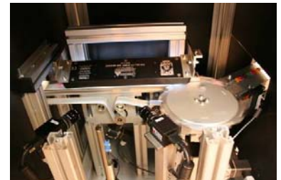
<< Inspection station with two individual OCR cameras mounted on opposite sides of a conveyor
