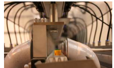
<< Components diverted into a chute relevant to each component
